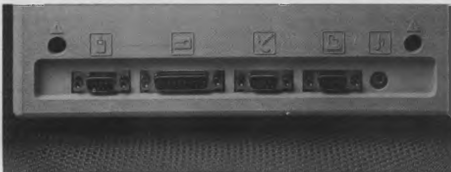
Above the interface ports are icons describing their respective functions
